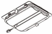
Streetlight 10 micro, LED module, primary light control with cycle path optic, light distribution: P1.0a, primary light characteristic: asymmetric, High Power LED, light colour: 750, colour temperature: 5000K, mains connection: 230..240V, 50Hz, LED module, length: 174mm, width: 137mm, height: 40mm, protection rating (complete): as luminaire, packaging unit: 1 piece
