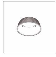
Highbay 42 S/L, reflector, primary light control with reflector, of PC, transparent prismatic structure, light emission: direct with ceiling illumination distribution, primary light characteristic: rotationally symmetric, installation type: surface-mounted, diameter: 410mm, height: 141mm, packaging unit: 1 piece
