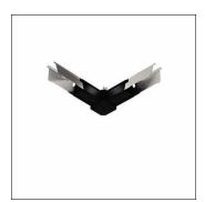
Licross®, L-connector, trunking rail element, of steel, galvanised, coated, matt jet black (RAL 9005), length: 197mm, width: 197mm, height: 67mm, blank cover, of PC/ABS, jet black (RAL 9005), connector, of steel, galvanised, protection rating (complete): for IP20/IP40 protection rating, certification: CE, UKCA, packaging unit: 1 piece
