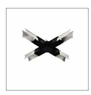
Licross®, X-connector, trunking rail element, of steel, galvanised, coated, matt jet black (RAL 9005), length: 300mm, width: 300mm, height: 67mm, blank cover, of PC/ABS, jet black (RAL 9005), connector, of steel, galvanised, protection rating (complete): for IP20/IP40 protection rating, certification: CE, UKCA, packaging unit: 1 piece
