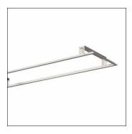
Sport 31, ceiling recessing frame, installation type: recessed, mounting frame, of sheet steel, traffic white (RAL 9016), incl. screws, length: 1.582mm, width: 458mm, height: 105mm, clamping range: 10..60mm, packaging unit: 1 piece
