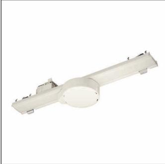
Licross®sensor D1, slave, central control - connection to lighting or building management, local control - self-sufficient standalone sensors, dimmable, installation type: recessed, installation location: to the Licross® trunking rail, of sheet steel, protection rating (complete): IP20, insulation class (complete): insulation class I (protective earthing), certification: CE, UKCA, voltage: 120..277V, voltage type: AC, 1 x light sensor, 1 x DALI-2, packaging unit: 1 piece
