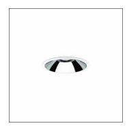
Lunis 21, L, downlight, of PC, light emission: direct distribution, LED rated luminous flux: 1.670lm, light colour: 830, control gear: ECG DALI, with terminal, 5-pole, mains connection: 220..240V, AC, housing, round, of diecast aluminium, traffic white (RAL 9016), diameter: 162mm, protection rating (complete): IP20, protection rating (on room side): IP54, insulation class (complete): insulation class II (safety insulation), certification: CE, impact resistance: IK02, packaging unit: 1 piece
