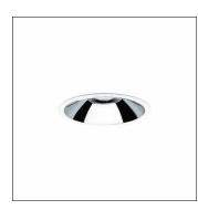
Lunis 21, XL, downlight, of PC, light emission: direct distribution, LED rated luminous flux: 2.180lm, light colour: 830, control gear: ECG, with terminal, 3-pole, mains connection: 220..240V, AC, housing, round, of diecast aluminium, traffic white (RAL 9016), diameter: 213mm, protection rating (complete): IP20, protection rating (on room side): IP54, insulation class (complete): insulation class II (safety insulation), certification: CE, impact resistance: IK02, packaging unit: 1 piece
