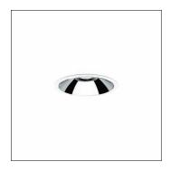
Lunis 21, L, downlight, of PC, light emission: direct distribution, LED rated luminous flux: 1.670lm, light colour: 830, control gear: ECG, with terminal, 3-pole, mains connection: 220..240V, AC, housing, round, of diecast aluminium, traffic white (RAL 9016), diameter: 162mm, protection rating (complete): IP20, protection rating (on room side): IP54, insulation class (complete): insulation class II (safety insulation), certification: CE, impact resistance: IK02, packaging unit: 1 piece
