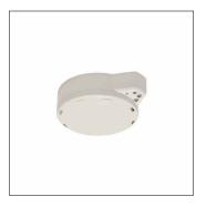
DALI2sensor D1, slave, central control - connection to lighting or building management, dimmable, installation type: surface-mounted, installation location: to the ceiling, of plastic, protection rating (complete): IP20, insulation class (complete): insulation class I (protective earthing), certification: CE, UKCA, voltage: 120..277V, voltage type: AC, 1 x light sensor, 1 x DALI-2, packaging unit: 1 piece
