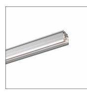
AX T, 3-phase track, installation type: suspended mounting, surface-mounted, control gear: ON/OFF, mains connection: 220..240V/380..400V, AC, of extruded aluminium section, coated, grey, length: 2.000mm, width: 32mm, height: 33mm, protection rating (complete): IP20, insulation class (complete): insulation class I (protective earthing), certification: CE, ENEC, packaging unit: 1 piece
