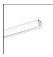
AX T, 3-phase track, installation type: suspended mounting, surface-mounted, control gear: ON/OFF, mains connection: 220..240V/380..400V, AC, of extruded aluminium section, coated, white, length: 1.000mm, width: 32mm, height: 33mm, protection rating (complete): IP20, insulation class (complete): insulation class I (protective earthing), certification: CE, ENEC, packaging unit: 1 piece
