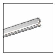
AX T, 3-phase track, installation type: suspended mounting, surface-mounted, control gear: DALI, mains connection: 220..240V/380..400V, AC, of extruded aluminium section, coated, grey, length: 3.000mm, width: 32mm, height: 33mm, protection rating (complete): IP20, insulation class (complete): insulation class I (protective earthing), certification: CE, ENEC, packaging unit: 1 piece
