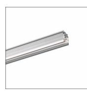
AX T, 3-phase track, installation type: suspended mounting, surface-mounted, control gear: DALI, mains connection: 220..240V/380..400V, AC, of extruded aluminium section, coated, grey, length: 2.000mm, width: 32mm, height: 33mm, protection rating (complete): IP20, insulation class (complete): insulation class I (protective earthing), certification: CE, ENEC, packaging unit: 1 piece
