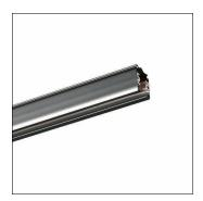
AX T, 3-phase track, installation type: suspended mounting, surface-mounted, control gear: ON/OFF, mains connection: 220..240V/380..400V, AC, of extruded aluminium section, coated, jet black (RAL 9005), length: 2.000mm, width: 32mm, height: 33mm, protection rating (complete): IP20, insulation class (complete): insulation class I (protective earthing), certification: CE, ENEC, packaging unit: 1 piece
