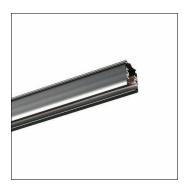
AX T, 3-phase track, installation type: suspended mounting, surface-mounted, control gear: DALI, mains connection: 220..240V/380..400V, AC, of extruded aluminium section, coated, jet black (RAL 9005), length: 1.000mm, width: 32mm, height: 33mm, protection rating (complete): IP20, insulation class (complete): insulation class I (protective earthing), certification: CE, ENEC, packaging unit: 1 piece
