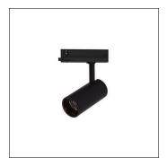
Spot 31 Slim, directional spotlight, light control with reflector, of aluminium, LED rated luminous flux: 2.150lm, light colour: 927, control gear: ECG, with 3-phase adapter, mains connection: 220..240V, AC, 50/60Hz, housing, of aluminium, jet black (RAL 9005), diameter: 70mm, adapter, of plastic, protection rating (complete): IP20, insulation class (complete): insulation class I (protective earthing), certification: CE, impact resistance: IK02, packaging unit: 1 piece
