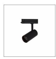
Spot 31 Slim, directional spotlight, light control with reflector, of aluminium, LED rated luminous flux: 2.100lm, light colour: 927, control gear: ECG, with 3-phase adapter, mains connection: 220..240V, AC, 50/60Hz, housing, of aluminium, jet black (RAL 9005), diameter: 70mm, adapter, of plastic, protection rating (complete): IP20, insulation class (complete): insulation class I (protective earthing), certification: CE, impact resistance: IK02, packaging unit: 1 piece
