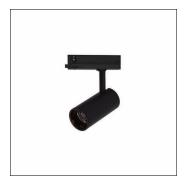
Spot 31 Slim, directional spotlight, light control with reflector, of aluminium, LED rated luminous flux: 2.200lm, light colour: 930, control gear: ECG, with 3-phase adapter, mains connection: 220..240V, AC, 50/60Hz, housing, of aluminium, jet black (RAL 9005), diameter: 70mm, adapter, of plastic, protection rating (complete): IP20, insulation class (complete): insulation class I (protective earthing), certification: CE, impact resistance: IK02, packaging unit: 1 piece
