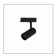
Spot 31 Slim, directional spotlight, light control with reflector, of aluminium, LED rated luminous flux: 2.150lm, light colour: 930, control gear: ECG, with 3-phase adapter, mains connection: 220..240V, AC, 50/60Hz, housing, of aluminium, jet black (RAL 9005), diameter: 70mm, adapter, of plastic, protection rating (complete): IP20, insulation class (complete): insulation class I (protective earthing), certification: CE, impact resistance: IK02, packaging unit: 1 piece
