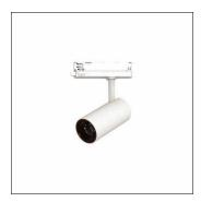
Spot 31 Slim, directional spotlight, light control with reflector, of aluminium, LED rated luminous flux: 2.150lm, light colour: 930, control gear: ECG, with 3-phase adapter, mains connection: 220..240V, AC, 50/60Hz, housing, of aluminium, traffic white (RAL 9016), diameter: 70mm, adapter, of plastic, protection rating (complete): IP20, insulation class (complete): insulation class I (protective earthing), certification: CE, impact resistance: IK02, packaging unit: 1 piece
