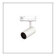
Spot 31 Slim, directional spotlight, light control with reflector, of aluminium, LED rated luminous flux: 2.100lm, light colour: 927, control gear: ECG, with 3-phase adapter, mains connection: 220..240V, AC, 50/60Hz, housing, of aluminium, traffic white (RAL 9016), diameter: 70mm, adapter, of plastic, protection rating (complete): IP20, insulation class (complete): insulation class I (protective earthing), certification: CE, impact resistance: IK02, packaging unit: 1 piece
