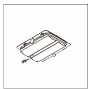
Streetlight 10 micro, LED module, light distribution: ST1.2a, primary light characteristic: asymmetric, High Power LED, light colour: 722, colour temperature: 2200K, mains connection: 230..240V, 50Hz, LED module, length: 174mm, width: 137mm, height: 40mm, protection rating (complete): as luminaire, packaging unit: 1 piece
