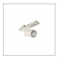
Licross® Spot 31, directional spotlight, light control with lens, of plastic, LED rated luminous flux: 5.250lm, light colour: 940, with plug, 3-pole, with phase selection, mains connection: 220..240V, AC, 50/60Hz, of aluminium, traffic white (RAL 9016), length: 140mm, diameter: 90mm, protection rating (complete): IP20, insulation class (complete): insulation class I (protective earthing), certification: CE, packaging unit: 1 piece
