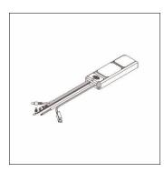
Lunis 21, emergency light element, EM-KIT 3h,with system connector: socket 2.1mm, rated input power: 3W, battery: LiFePO4, 2,2Ah, housing, of plastic, white, length: 212mm, width: 73mm, height: 28mm, protection rating (complete): IP20, insulation class (complete): insulation class II (safety insulation), certification: CE, impact resistance: IK02, permissible operating ambient temperature: 0..+50°C, packaging unit: 1 piece
