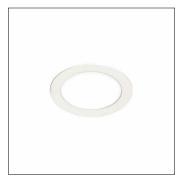
Lunis 41, Flat, downlight, light emission: direct distribution, LED rated luminous flux: 2.360lm, light colour: 830/840, mains connection: 230V, AC, 50/60Hz, housing, round, of aluminium, coated, traffic white (RAL 9016), diameter: 225mm, protection rating (complete): IP20, protection rating (on room side): IP44, insulation class (complete): insulation class II (safety insulation), certification: CE, permissible ambient temperature for indoor applications: -20..+40°C, packaging unit: 1 piece
