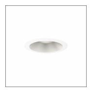
Lunis 31, -XL, downlight, light control with lens, light emission: direct distribution, LED rated luminous flux: 2.500lm, light colour: 840, mains connection: 220..240V, AC/DC, 0/50..60Hz, housing, of aluminium, white, protection rating (complete): IP20, protection rating (on room side): IP54, insulation class (complete): insulation class II (safety insulation), certification: CE, ENEC, packaging unit: 1 piece
