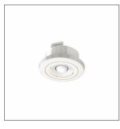
SITECO Connect 11H WirelessNode Environment Sensor, slave, local control-self-sufficient standalone sensors, dimmable, installation type: recessed, installation location: in the ceiling, of plastic, protection rating (complete): IP20, certification: CE, UKCA, 1 x PIR movement sensor, 1 x light sensor, 1 x DALI, 1 x Bluetooth® interface, packaging unit: 1 piece
