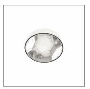
SITECO Connect 11H Wireless, surface-mounted housing, installation type: surface-mounted, control gear: Bluetooth® Mesh, housing, of plastic, white, diameter: 105mm, height: 25mm, surface-mounted housing, local control - self-sufficient standalone sensors, dimmable, protection rating (complete): IP54, certification: CE, UKCA, permissible operating ambient temperature: 0..+50°C, packaging unit: 1 piece
