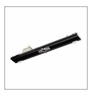
Licross®, rail insert, adapter,with plug, 5-pole, with phase selection, mains connection: 230V, AC, 50/60Hz, terminal,5-pole, max. 2.5mm², multi adapter, of sheet steel, coil coated, matt jet black (RAL 9005), for IP20/IP40 protection rating, length: 500mm, width: 64mm, height: 68mm, multifunctional insert, protection rating (complete): IP20, insulation class (complete): insulation class I (protective earthing), certification: CE, UKCA, packaging unit: 1 piece
