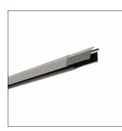
Licross<sup>®</sup>, trunking rail, of sheet steel, galvanised, coil coated, metallic grey (RAL 9006), length: 4.500 mm, width: 64 mm, height: 67mm, protection rating (complete): maximum IP64, depends on used inserts and accessories, insulation class (complete): insulation class I (protective earthing), certification: CE, UKCA, LABS conformity tested according to VDMA 24364:2018-05, packaging unit: 1 piece
