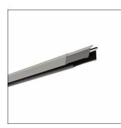
Licross<sup>®</sup>, trunking rail, of sheet steel, galvanised, coil coated, metallic grey (RAL 9006), length: 1.500 mm, width: 64 mm, height: 67mm, through-wiring: 14x 2.5mm<sup>2</sup>, protection rating (complete): maximum IP64, depends on used inserts and accessories, insulation class (complete): insulation class I (protective earthing), certification: CE, UKCA, LABS conformity tested according to VDMA 24364:2018-05, packaging unit: 1 piece
