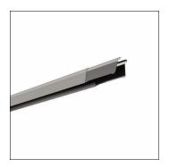
Licross®, trunking rail, of sheet steel, galvanised, coil coated, metallic grey (RAL 9006), length: 3.000 mm, width: 64 mm, height: 67mm, through-wiring: 14x 2.5mm², protection rating (complete): maximum IP64, depends on used inserts and accessories, insulation class (complete): insulation class I (protective earthing), certification: CE, UKCA, LABS conformity tested according to VDMA 24364:2018-05, packaging unit: 1 piece
