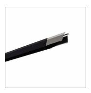
Licross®, trunking rail, of sheet steel, galvanised, coil coated, matt jet black (RAL 9005), length: 1.500 mm, width: 64 mm, height: 67mm, through-wiring: 14x 2.5mm², protection rating (complete): maximum IP64, depends on used inserts and accessories, insulation class (complete): insulation class I (protective earthing), certification: CE, UKCA, LABS conformity tested according to VDMA 24364:2018-05, packaging unit: 1 piece
