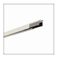
Licross®, trunking rail, of sheet steel, galvanised, coil coated, white, length: 4.500 mm, width: 64 mm, height: 67mm, through-wiring: 14x 2.5mm², protection rating (complete): maximum IP64, depends on used inserts and accessories, insulation class (complete): insulation class I (protective earthing), certification: CE, UKCA, LABS conformity tested according to VDMA 24364:2018-05, packaging unit: 1 piece
