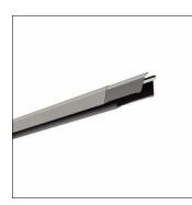
Licross<sup>®</sup>, trunking rail, of sheet steel, galvanised, coil coated, metallic grey (RAL 9006), length: 1.500 mm, width: 64 mm, height: 67mm, through-wiring: 7x 2.5mm<sup>2</sup>, protection rating (complete): maximum IP64, depends on used inserts and accessories, insulation class (complete): insulation class I (protective earthing), certification: CE, UKCA, LABS conformity tested according to VDMA 24364:2018-05, packaging unit: 1 piece
