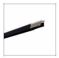
Licross®, trunking rail, of sheet steel, galvanised, coil coated, matt jet black (RAL 9005), length: 3.000 mm, width: 64 mm, height: 67mm, through-wiring: 7x 2.5mm², protection rating (complete): maximum IP64, depends on used inserts and accessories, insulation class (complete): insulation class I (protective earthing), certification: CE, UKCA, LABS conformity tested according to VDMA 24364:2018-05, packaging unit: 1 piece
