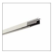
Licross®, trunking rail, of sheet steel, galvanised, coil coated, white, length: 3.000 mm, width: 64 mm, height: 67mm, protection rating (complete): maximum IP64, depends on used inserts and accessories, insulation class (complete): insulation class I (protective earthing), certification: CE, UKCA, LABS conformity tested according to VDMA 24364:2018-05, packaging unit: 1 piece
