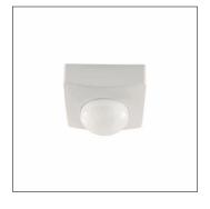
SITECO ConnectSensor-Head PR1-S, slave, local control - self-sufficient standalone sensors, central control - connection to lighting or building management, dimmable, installation type: slip-in mounting, installation location: to the ceiling, to the Modario® trunking rail, to the Licross® trunking rail, of plastic, protection rating (complete): IP54, certification: CE, VDE, 1 x PIR movement sensor, 1 x light sensor, packaging unit: 1 piece
