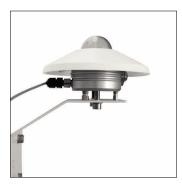
iLuxsensor, installation type: surface-mounted, installation location: to the wall, to mast, of diecast aluminium, protection rating (complete): IP65, insulation class (complete): insulation class II (safety insulation), certification: CE, connection cable included, cable length: 10 m, 1 x illuminance, 1 x serial interface, 1 x digital TTL level, packaging unit: 1 piece
