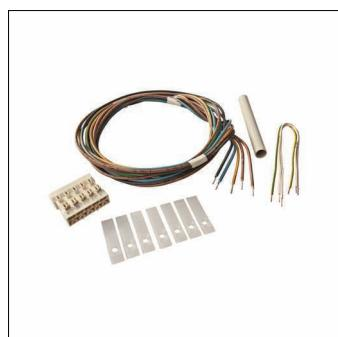
Monsun 21 Gen.1, through-wiring, installation type: recessed, through-wiring set, 5-core, 1.5mm<sup>2</sup>, cable length: 1.6m, terminal, 5-pole, max. 2.5mm<sup>2</sup>, with protective earth, insulation class (complete): insulation class I (protective earthing), packaging unit: 1 piece
