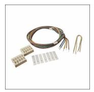
Monsun® 21 Gen.1, through-wiring, installation type: recessed, through-wiring set,5-core, 1.5mm², cable length: 1,4m, terminal,5-pole, max. 2.5mm², with protective earth, insulation class (complete): insulation class I (protective earthing), packaging unit: 1 piece
