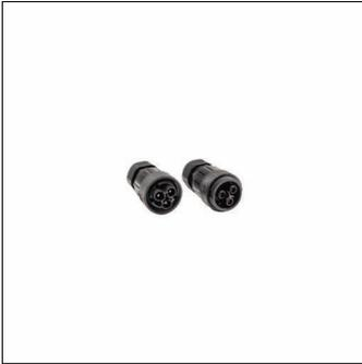
plug connection, system connector: plug/socket,3-pole, max. 2.5mm<sup>2</sup>, cable infeed: 8mm, of PC, black, protection rating (complete): IP65, packaging unit: 1 piece
