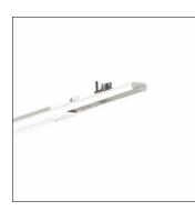
Modario<sup>®</sup>, track adapter insert, with plug, 5-pole, with phase selection, for trunking rail, 5 or 10-core, mains connection: 230/400V, track adapter insert, of sheet steel, coil coated, pure white, 2x system unit, max. weight load 5kg, length: 598mm, width: 48mm, protection rating (complete): for IP20 protection rating, insulation class (complete): insulation class I (protective earthing), certification: CE, packaging unit: 1 piece
