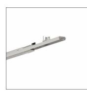
Modario<sup>®</sup>, track adapter insert, control gear: DALI, with plug, 5-pole, with phase selection, for trunking rail, 10-core, mains connection: 230/400V, track adapter insert, of sheet steel, coil coated, metallic grey (RAL 9006), 4x system unit, max. weight load 5kg, length: 1.196mm, width: 48mm, protection rating (complete): for IP20 protection rating, insulation class (complete): insulation class I (protective earthing), certification: CE, packaging unit: 1 piece
