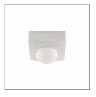
SITECO ConnectSensor-Head PC5-S, slave, local control - self-sufficient standalone sensors, central control - connection to lighting or building management, dimmable, installation type: slip-in mounting, installation location: to the ceiling, to the Modario® trunking rail, to the Licross® trunking rail, of plastic, protection rating (complete): IP54, certification: CE, VDE, 1 x PIR movement sensor, 1 x light sensor, packaging unit: 1 piece
