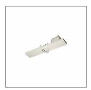
Licross®sensor PC3, slave, central control - connection to lighting or building management, dimmable, installation type: recessed, installation location: to the Licross® trunking rail, of sheet steel, protection rating (complete): IP20, insulation class (complete): insulation class I (protective earthing), certification: CE, UKCA, 1 x PIR movement sensor, 1 x light sensor, 1 x DALI-2, packaging unit: 1 piece
