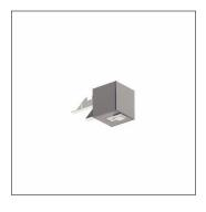
Silica® 21sensor module PR3-S, slave, central control, dimmable, installation arrangement: single/continuous arrangement, installation type: slip-in mounting, installation location: to the luminaire, of extruded aluminium section, protection rating (complete): IP20, insulation class (complete): insulation class I (protective earthing), certification: CE, 1 x PIR movement sensor, 1 x light sensor, packaging unit: 1 piece
