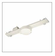
Licross®light sensor D1, slave, central control - connection to lighting or building management, local control - self-sufficient standalone sensors, dimmable, installation location: to the Licross® trunking rail, of sheet steel, protection rating (complete): IP20, insulation class (complete): insulation class I (protective earthing), certification: CE, UKCA, voltage: 120..277V, voltage type: AC, 1 x light sensor, 1 x DALI-2, packaging unit: 1 piece
