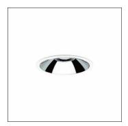
Lunis 21, XL, downlight, of PC, light emission: direct distribution, LED rated luminous flux: 2.280lm, light colour: 840, control gear: ECG DALI, with terminal, 5-pole, mains connection: 220..240V, AC, housing, round, of diecast aluminium, traffic white (RAL 9016), diameter: 213mm, protection rating (complete): IP20, protection rating (on room side): IP54, insulation class (complete): insulation class II (safety insulation), certification: CE, impact resistance: IK02, packaging unit: 1 piece
